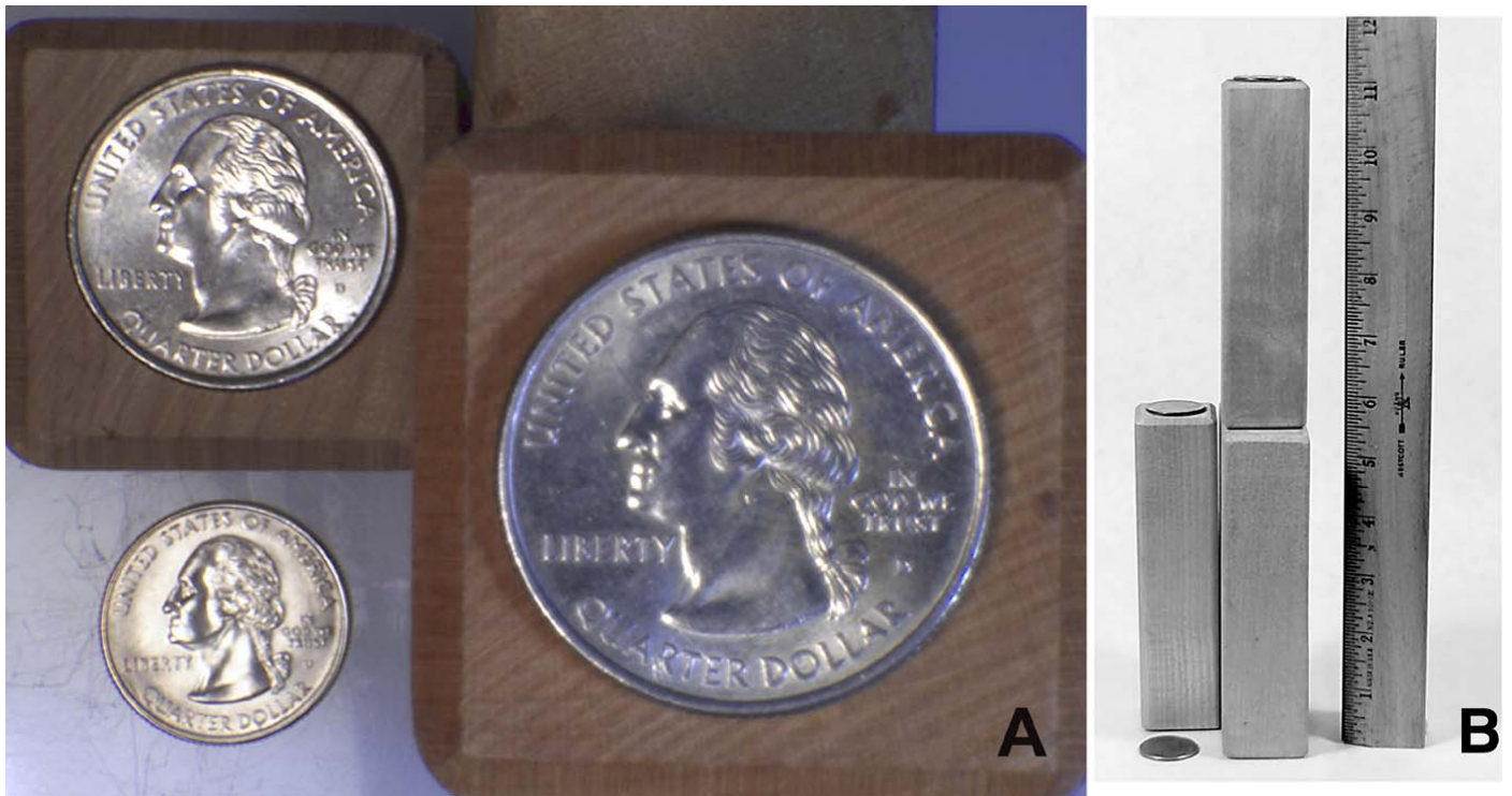
Figure 5. A: Image taken with a 600CL of US quarters on blocks of wood. The image was levels adjusted and sharpened in Adobe Photoshop. The camera was focused on the middle quarter with the Computar iris at f 5.6 and the image taken at an f -stop slightly above “+” (i.e., more than one f -stop above 32, see Fig. 4). Image depth of field/field width is approximately 3.5. B: Side view of the same objects shown in A. Approximately 140 mm (5 ½ inches) separate each quarter for a total depth of field of more than 280 mm (11 inches).
